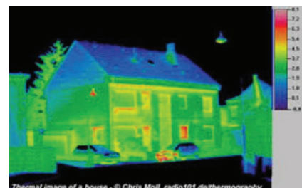
Image of a well insulated building, with minimal thermal leakage
